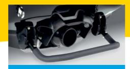
Rear Boarding Step A standard feature on the F-12X GPScape, this makes getting back up on the boat easier than ever. It's also available as an accessory for the F-12X and F-12.
